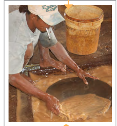
RECOVERY OF SLURRY LADEN WITH MERCURY
