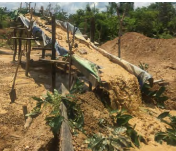
Miners using hydraulic pump – soil sediments going straight to the launder © 2016 Evelyn Cubelo / BAN Toxics
