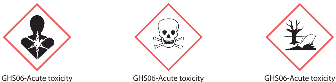
Figure 5 GHS hazard pictograms for mercury wastes 45
